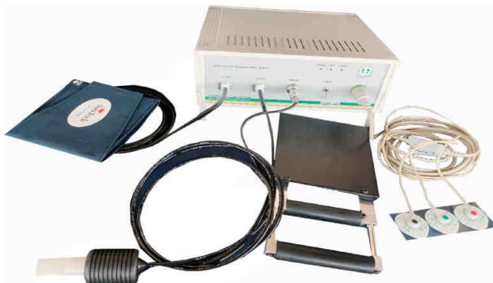
Fig. 1. The computerized autonomic neuropathy analyser (CANS 504).
